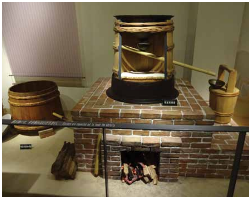
Kabuto Pot Still made of wood, were used for distillation in old Japan, from the Edo to Meiji Periods. The same wooden types are still used today in Southeast Asia.
